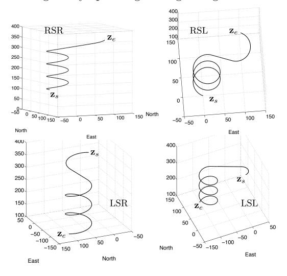
Medium altitude case:  $L_{\rm car}(R_{\rm min})\tan\bar{\gamma} < |z_{de} - z_{ds}| \le [L_{\rm car}(R_{\rm min}) + 2\pi R_{\rm min}]\tan\bar{\gamma}$  To achieve altitude gain, must add path deviation.
